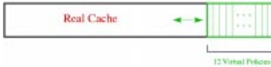
Figure 3: Virtual caches embedded in the cache memory.
